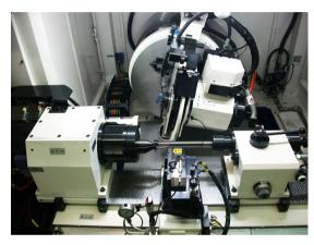
• Moving-head cross slide configuration. L > 3000 mm RER-SP Model
